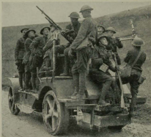
Tender of an Observation Balloon Mounted with Two Machine Guns for Anti-Aircraft Defense
