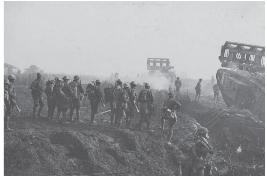
American soldiers advance with tanks near Bellicourt on September 29, 1918. The frames atop the tanks are for dropping in trenches to aid crossing.
